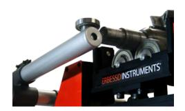
Designed to limit the axial rotor's displacement on the EI-1000 balancing machine. It has 2 axes to adjust up to 1 meter shaft's length from the supports. They include the mounting base to the balancing pedestal, an axial and radial arm and a rolling element at the tip. EI-1000 includes 2 axial supports.
