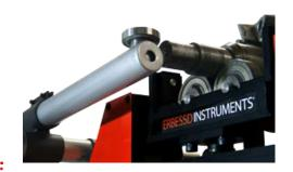
Designed to limit the axial rotor's displacement on the EI-4500 balancing machine. It has 2 axes to adjust up to 1 meter shaft's length from the supports. They include the mounting base to the balancing pedestal, an axial and radial arm and a rolling element at the tip. EI-4500 includes 2 axial supports.
