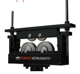
It's an accessory for El-4500 balancing machine required when rotors are mounted on cantilever and/ortosecurerotors with high levels of vibration, like crankshafts. Each support includes bearings and has adjustable height. Its dimensions may vary depending on the bearing suspensions. Sold separately.
