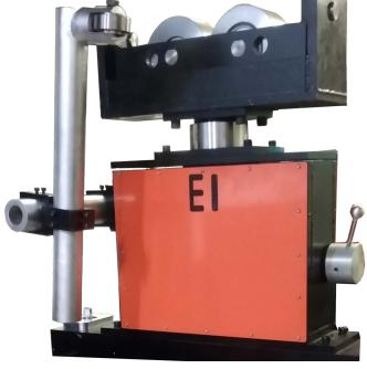
The El-4500 can support up to 4 500 kg (2,250 kg each support) and with its 2 roller positions it allows shaft diameters of 279.4 mm (11 in). It also has an elevator screw to adjust the position in case the tracks rotor supports have different diameters up to 50.8 mm (2 in) and a swinging movement for autoalignment.
