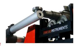
Designed to limit the axial rotor's displacement on the EI-6000 balancing machine. It has 2 axes to adjust up to 1 meter shaft's length from the supports. They include the mounting base to the balancing pedestal, an axial and radial arm and a rolling element at the tip. EI-6000 includes 2 axial supports.
